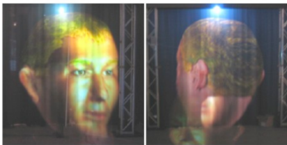
(Figure 2, support for dual-sided projection allows two independent images to be projected on each side, such that a 3D application can render two interactive views for a pseudo-3D effect (Olwal et al., 2006))
